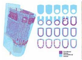
Model cross sections at 3D biological shield model different heights
