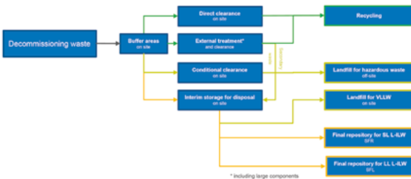
Figure 1: available waste routes in Sweden, including SKB's geological repositories SFR and SFL (planned).
